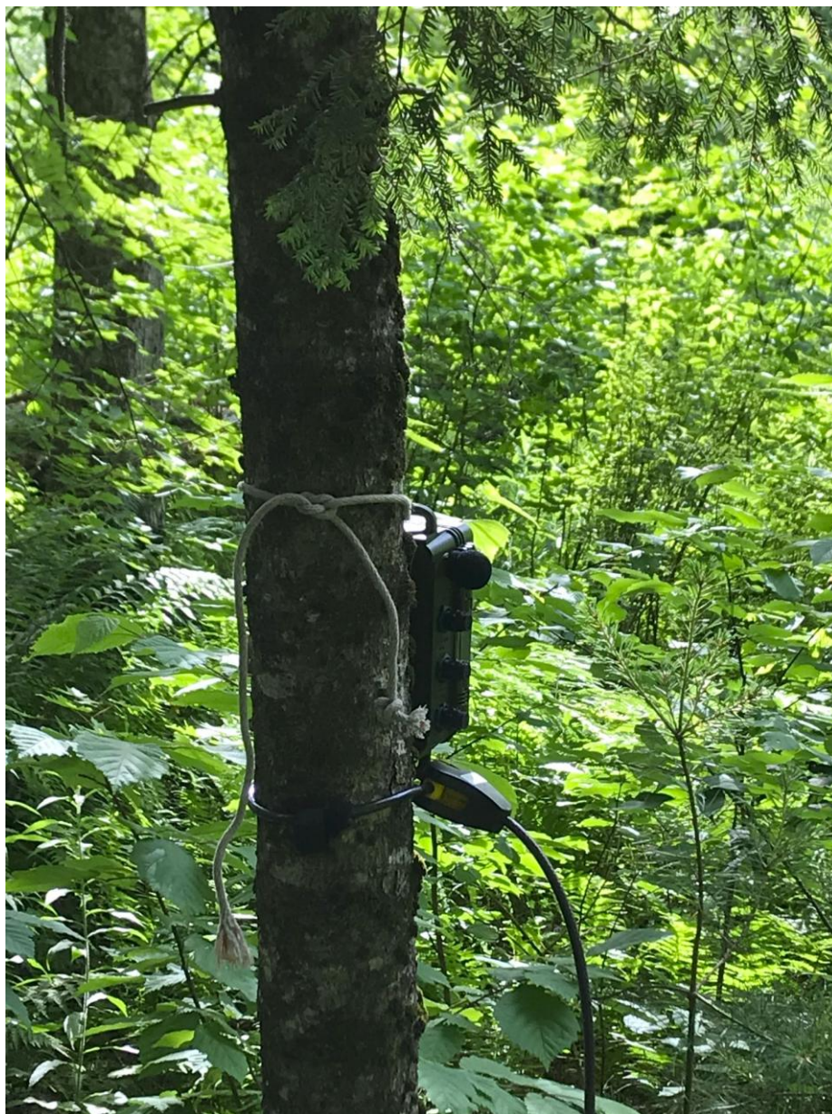
An autonomous recording unit attached and locked to a tree, ready to begin recording following sunset. © Ben Fletcher
